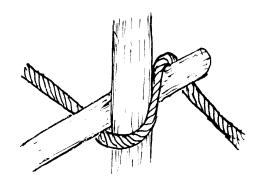
**STEP 3:** While one person holds the up right pole, a second person rotates the longer pole around the upright so that the rope begins to wrap around the upright pole. Adjust the height of the rope so that it can be easily stepped over.
