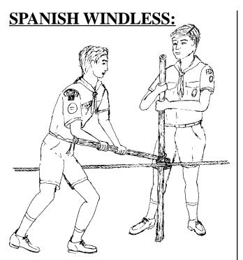
A Spanish windless is a device for moving heavy loads such as rocks and logs.
