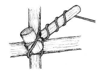
The dovetail maul makes a good rope wrench. Pass the rope over the head of the maul and then take several wraps around the handle. The rope is then tightened by rotating the maul so that the rope wraps part way around the head of the maul.
