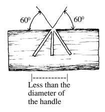
**[NOTE]** The width of the bottom of the dovetail notch must be less than the diameter of the handle.
