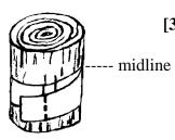
[3A] Wrap a strip of paper around the maul head. Cut the strip of paper off so that the two ends just meet.
