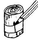
**STEP 4:** Drill handle hole in head. Use a 1 1/4 inch drill bit to drill a hole halfway through the head from one side, then finish drilling the hole from the other side of the maul head.
