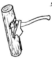
**STEP 1:** Use an ax to rough out the maul. Form a handle by cutting away one end of the piece of wood so that it is about 1 1/4 inches in diameter. Leave 4 to 5 inches of the other end at its original diameter to form the head of the maul.
