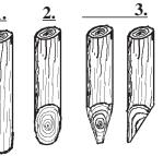
[Step 1] Cut to size. Length --- slightly longer than the width of the round lashing. Diameter --slightly larger than the gap formed between the rope, the flag pole, and the cleat.
